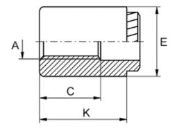
Female thread A = M2 Height K = 24 Hole diameter +0.1 = 3.7 Min distance to edge = 2.2 Min material thickness = 1.5 Outer diameter E = 6 Thread length = 9
